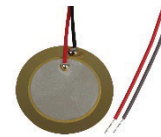
Piezoelectric material Applying electricity causes movement. Applying movement produces electricity
