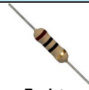
Resistor This limits the electrical current flowing through the circuit.
