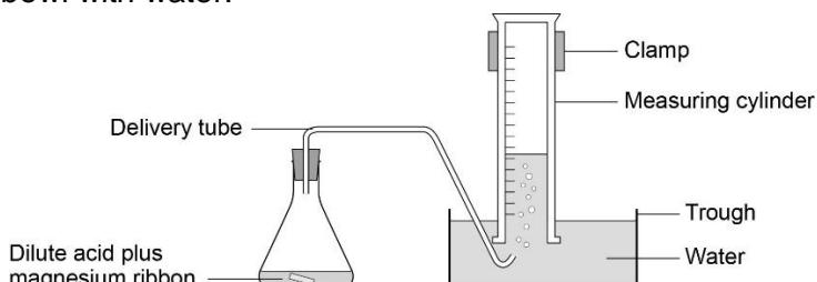
3. Fill the other measuring cylinder with water. Make sure it stays filled with water when you turn it upside down.
