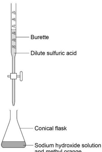
4. Put 5–10 drops of methyl orange indicator into the conical flask. Swirl to mix and place under the burette with the tile.
