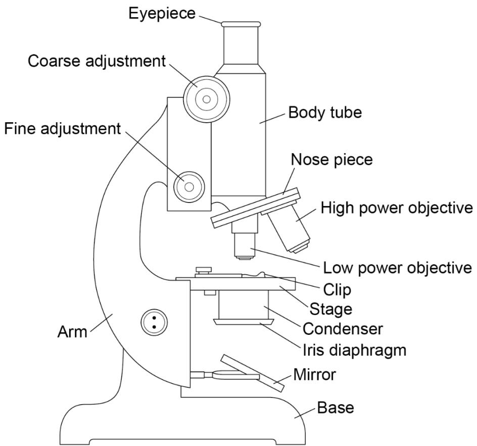
This microscope has a mirror to reflect light up through the slide. Some microscopes have a built-in light instead of a mirror.
